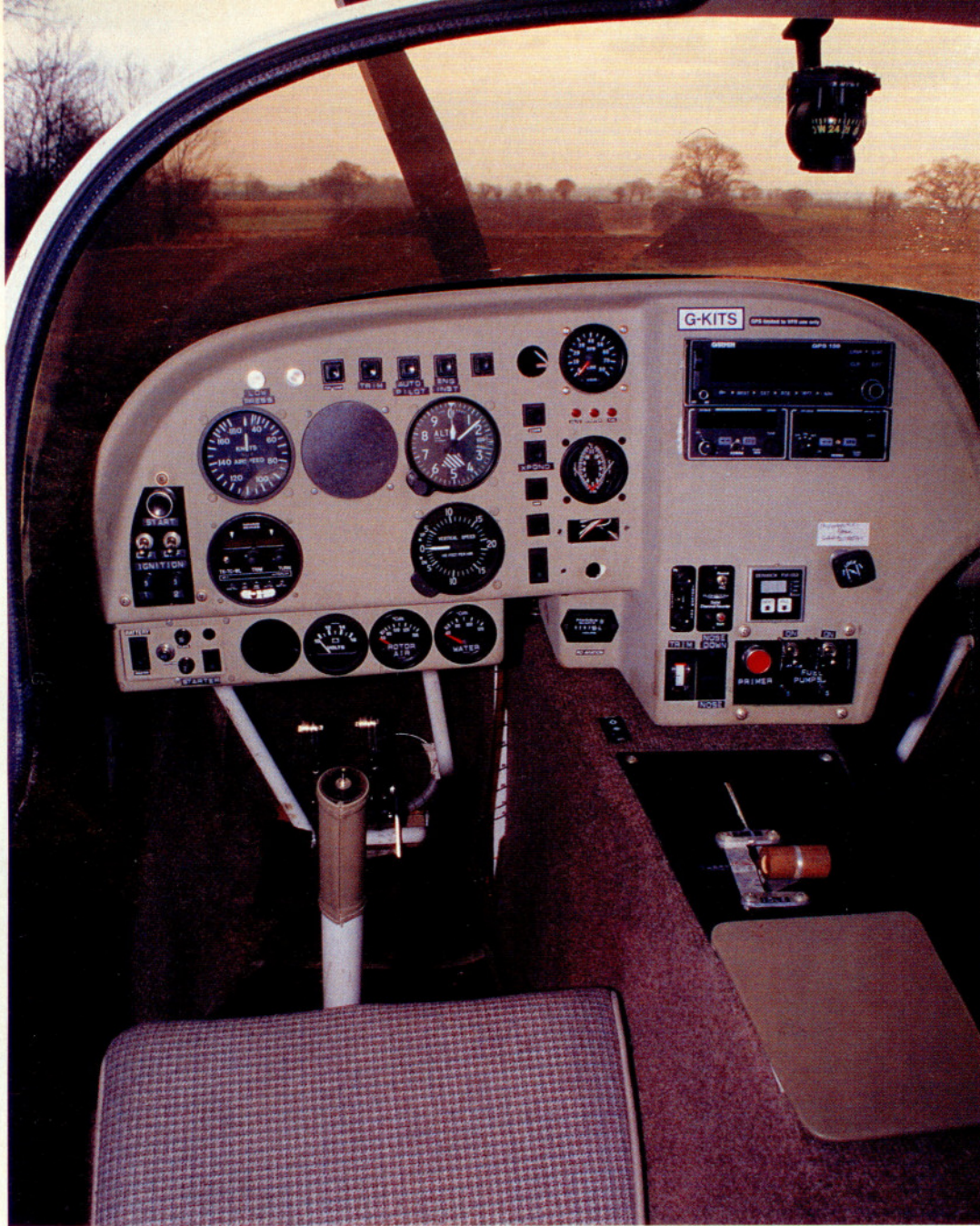
The tricycle-gear Europa uses the same one-piece molded instrument panel as its monowheel sibling (left). The selection of instruments and avionics is left to the builder.
