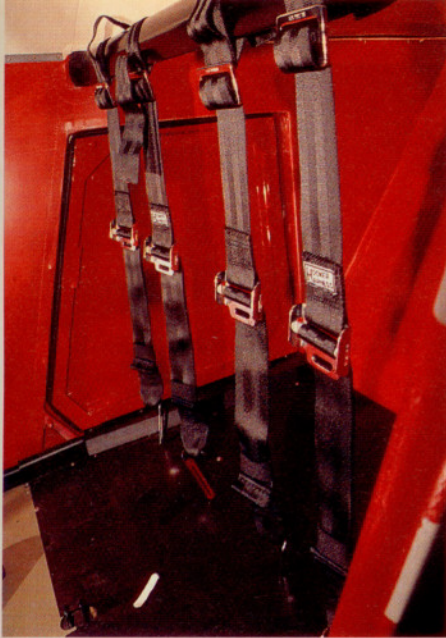
Repainting was necessary on only the cowling and wings (above right). After the off-airport excursion, four-point safety harnesses were installed at each of the four seating positions.
